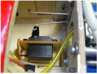
5. Finish the servo installation with two additional mounting screws.
