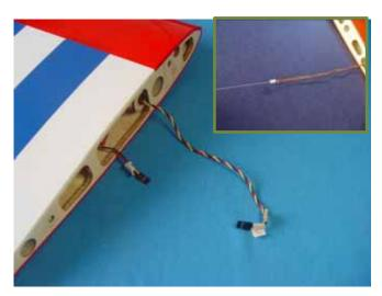
5. Use a 1mm drill bit to drill for the servo mounting screws. Install servo with output shaft toward the leading edge of the wing.
