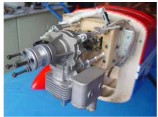
Note: Use Blue Loctite on final installation of engine mounting screws.
