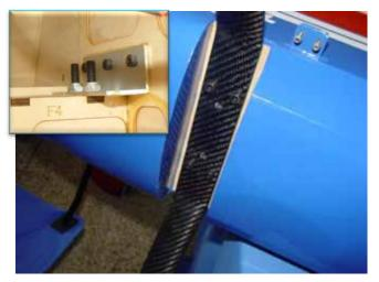
2. Install the landing gear axles with lock nut.
