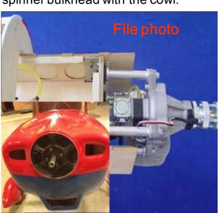
3. Remove cowl and mount fire wall at present location. Drill 3mm mounting holes for hardware through the motor box into aluminum angle brackets.
