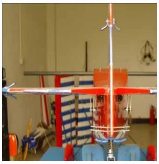
2. Attach the nylon clevises and threaded cable ends to the metal tail brackets. Install the included cables and crimp into position. Balance cable tensions.
