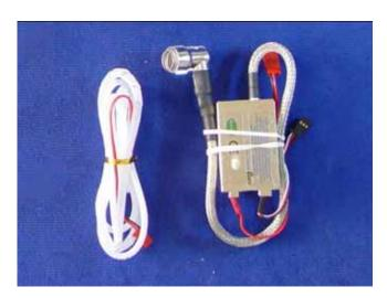
1. Attach foam rubber to the bottom of ignition with double sided tape and install spiral wrap cover to ignition lead as shown.
