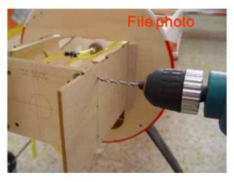
4. Glue the firewall at that location with 30 minute epoxy. Triangle stock is included to reinforce firewall.
