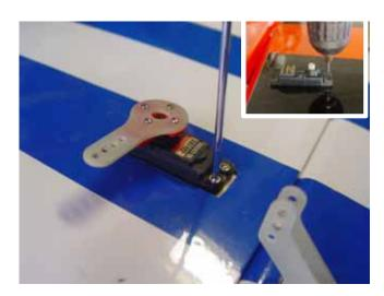
6. Install the servo arm facing outboard toward the wing tip. Adjust pushrod length so the servo arm is at 90 degrees and aileron panel in neutral position.
