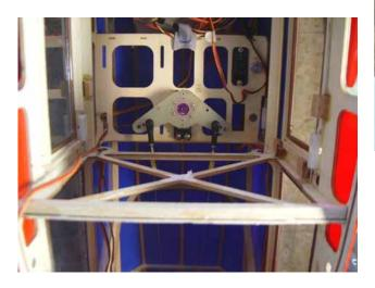
5. The flat surface of the ball link gets screwed against the servo arm.
