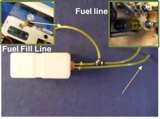
Mount the fuel tank with Velcro straps. There is a factory laser cut hole for the fueling dot aft of the engine cowl on the left hand side of the fuselage. Secure all fuel lines connections with zip ties.
