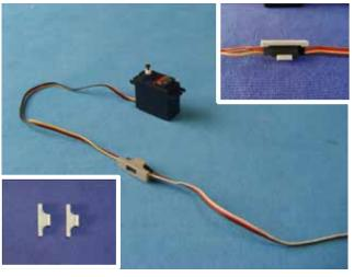
3. Locate servo cut outs and remove the covering with a knife. Tape the servo lead securely to the pull-string.
