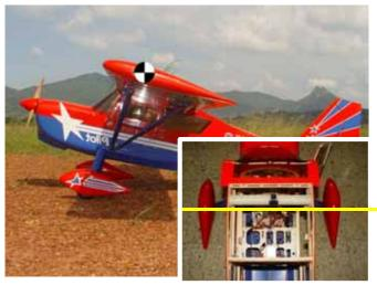
Avoid adding weight to your Decathlon for CG purposes. Position the batteries where required in order to correctly balance your model. Mount batteries on a bed of foam and secure with Nylon ties or Velcro straps.
