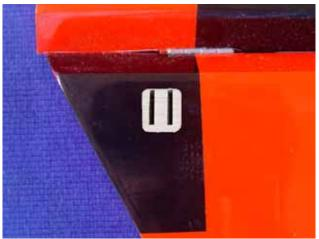
1. Tear off the cover on the horns and 3. Scuff the horns with a piece of locking plates sand paper for good glue bond. Wipe off sanding dust prior to gluing.
