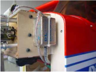
3. The ignition battery installs the same manor except under the engine box. Lock the connectors with the provided safety clip to prevent vibration from loosening connections.
