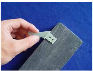
4. Apply 30 minutes epoxy inside the pre-cut slot for horn, and coat the horn with epoxy as shown.
