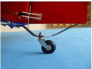
5. Drill a 1mm hole in the bottom of the rudder and mount steering spring with a wood screw as shown. Cut off excess wire from the spring.
