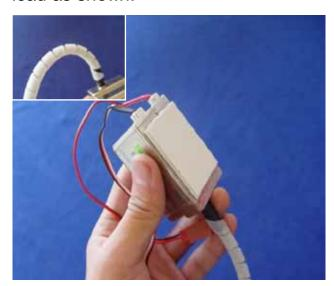
2. Stick the ignition to the outside of the engine box with double sided tape. Allow room for spark plug leads and wire connections. Drill holes in motor box for zip ties and secure module with ties.
