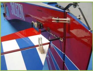
5. Install the stab with mounting bolts and washers. Apply Loctite to threads before installation.
