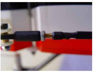
8. Shrink the heat shrinking tube over the crimp for a clean appearance.
