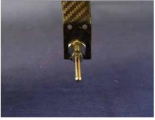
4. Install wheels and wheel collars using **Blue Loctite** on the set screws.
