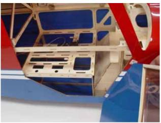
Note: Factory installed laser cut switch mounting holes are located under the covering on either side of the fuselage for your convenience.
