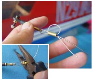
7. This is what a completed cable should look like. Cut off excess cable after crimping. Repeat process for opposite rudder cable.
