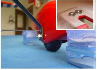
3. Finish the wheel pant mounting with the bolts and use Blue Loctite on the threads.
