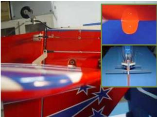
6. Install the servo arm facing down. Adjust pushrod length so the elevator is neutral and the servo horn is at 90 degrees.
