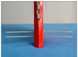
5. Slide the horn into slots with locking mount plates. Wipe away excess glue with rubbing alcohol.
