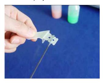
5. Slide the horn with locking plate into place. Wipe away excess epoxy with rubbing alcohol. Note: Some trimming of the horn might be required for the horn to fit flush.
