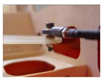
5. Install ball link to rudder control horn temporarily.
