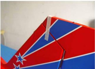
4. Mount the cables with the preinstalled ball link cable ends to the rudder servo arm. Cut the covering in the tail to expose cable exit slots. Run the cables out the slots. Make sure the cables cross in the middle.
