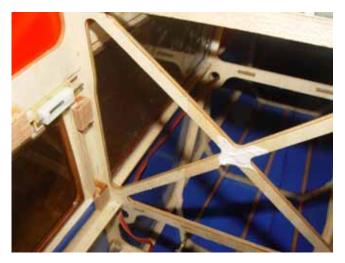
3. Use 1mm bit to drill the mounting holes. Install the servos with the out put shaft facing forward.
