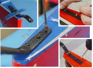
3. Install the blind nuts through the opening in the rear of the fuselage. Mount the tail wheel assembly using blue Loctite on the threads screws.
