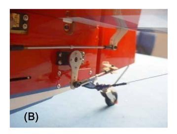
Pick the rudder servo mounting location based on CG needs.
