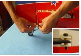
6. Prior to connecting rudder cable to the ball link, slide a section of heat shrink tubing and copper tubing. Run cable as shown looping around tubing. Remove excess slack from cable and crimp with diagonal pliers.
