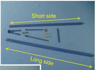
1. Install the brackets at mounting locations under side of wing. Use Loctite on threads.
