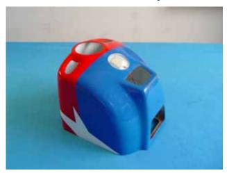
1. Use a Dremel cutting tool to rough cut the cowl for clearance for the exhaust system and for additional cooling. The air exit hole must be larger in diameter then the air inlet for sufficient cooling. Remove any rough edges with sandpaper.
