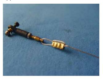
9. Adjust the rudder cable threaded fair leads to obtain appropriate cable tensions. Remove tape that was holding rudder straight.
