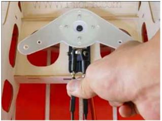
1. Drill 1mm holes and mount the rudder servo with the output shaft facing forward.
