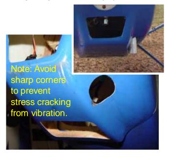
2. Install the plastic cooling air deflector(only offer for 107-122" decathlon) to the inside of the cowl. Secure with thick CA or silicone. Some trimming might be necessary for clearance with the engine.
