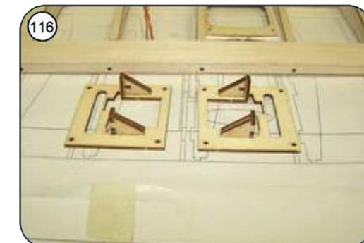
Install coverings F10 for the servo mounts and glue it on with wood glue.
