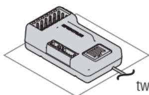
Mount the receiver flat, two possibilities are shown here
