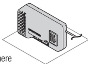
You may mount the receiver on any of its six sides, and it does not matter which direction the receiver is pointed. The receiver doesn't even need to be square with the vehicle, as long as it is flat and level.
