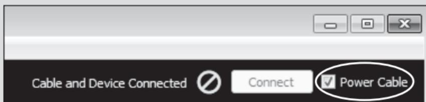
Make sure this check-box is checked to power the receiver from the PC during the update.
