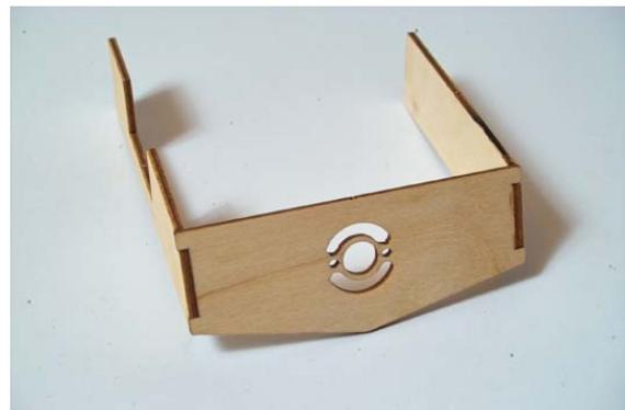
Now make the battery and receiver tray with parts 19, 20 and 21.
