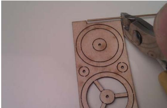
Use the cut out on the laser sheet to cut equal lengths for 6 spokes from the brass wire 1 mm.
