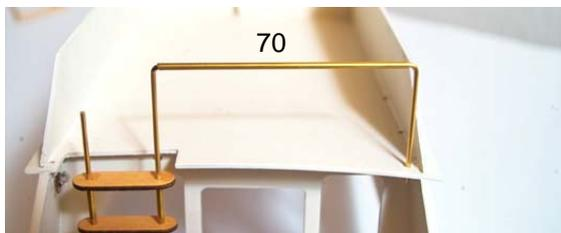
Make the lower rail from two split pins (71) and the tube (70).
