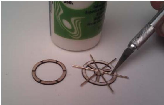
Apply some glue to the outer ring and into the center of the wheel and place the spokes carefully that they are lying up to the center hole, but leave it free.
