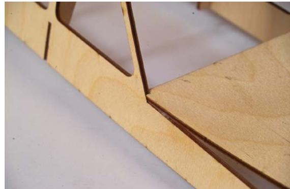
Try fit the parts first without glue. If necessary sand the slots or tenons for a perfect fit. Now first glue the side walls to the frame and back wall. When the gluing points are dry you can glue the bar (40) in place.
