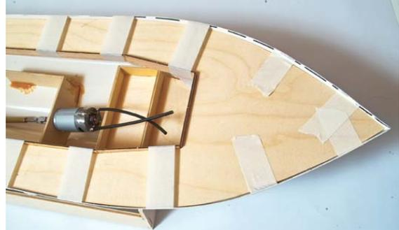
Fix the deck at several points with thin superglue. After that you can fix the deck complete with medium superglue. A good help is also Activator spray to shorten the drying process.
