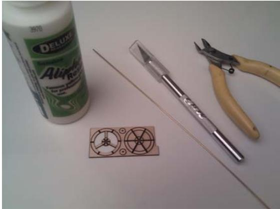
For this assembly for the steering wheel you will need the small laser sheet, 12 cm of brass wire 1 mm, and white glue or Aliphatic glue, a modelling knife, a wire cutter and some sand paper.
