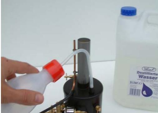
For producing steam you need water. That the water will not calcify your boiler, you should use distilled water only, which should be combined with 3-5% normal water to make it less aggressive. You can also use filtered rain water or water from the condenser of your tumble dryer.
