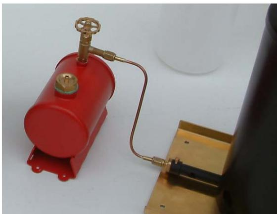
The tube of the burner looks out under the boiler at the front side. Connect the thin gas tube with two nuts to this thread. For tightening of the thread please use thread lock (Order No. 80474). Before that the tube must be bent to the gas tank fitting. If the tube is too long you can bend the tube like a coil around a round material of minimum 20 mm diameter. The longer tube helps that the boiler will not receive fluid gas.
