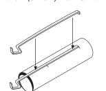
C. Insert the Engine Hook into the slit as shown.
