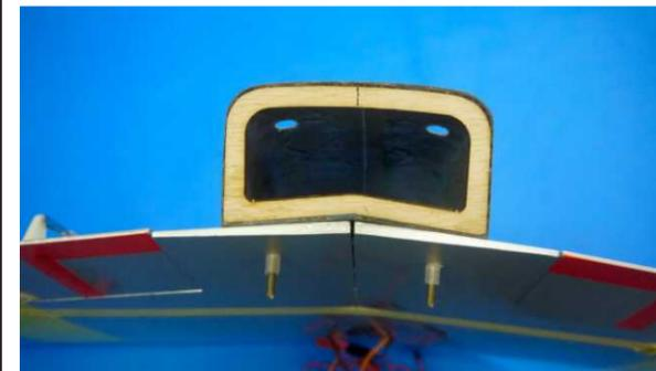
Insert the silicone tube to the end of wing bolt.
