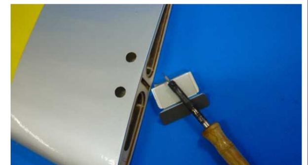
Try to find the exit hole for the servo line on the main wing. Remove the covering out of the hole.
