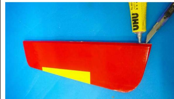
Try to find the slot on the rudder for installing the tail gear. Use sharp hobby knife to remove the covering out of the slot. Spread UHU glue or epoxy into the slot.
