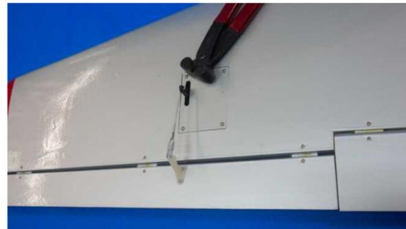
Thread the clip to the rod. Slide one piece of 5mm silicone tube to the connection of the control horn and clip. Use Z-bender to make a Z bend on the rod for connecting with servo arm.
