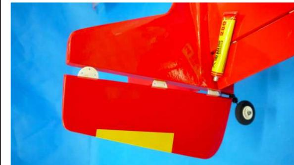
Spread Super glue on the one half of hinges and insert the hinges to the hinge slots on the rudder. Spread Super glue on the other half of hinges and insert the hinges to the slots on the vertical.
