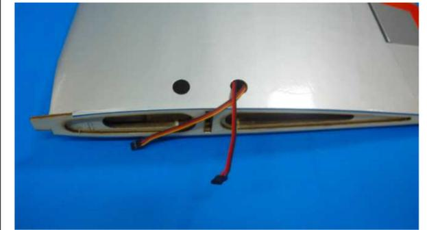
Pull the servo line out of the exit hole.
