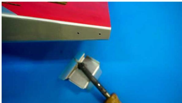
Place the fuselage upside down. Try to find the screw holes for the tail gear mount. Remove the covering out of the screw holes.
