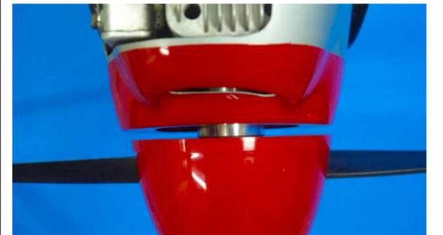
Assemble the spinner with propeller. Install the spinner to the motor. Please keep the distant between spinner and cowl around 2mm.
