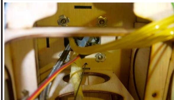
Push the claws nails to the holes inside the fuselage. It's better to use the engine screw M4x30 hex screw to secure the claws nails hard into the planking. Drop instant glue around the claws nail for securing it in place. Don't let the instant glue touch the screw.
