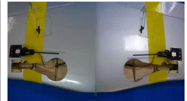
Place the main wing upside down. Try to find the Y-harness from the main gear mount. Plug the Y-harness and apply some transparent tape around the plug. Assemble the retracts on the main wing with M3x12 tapping screws.
