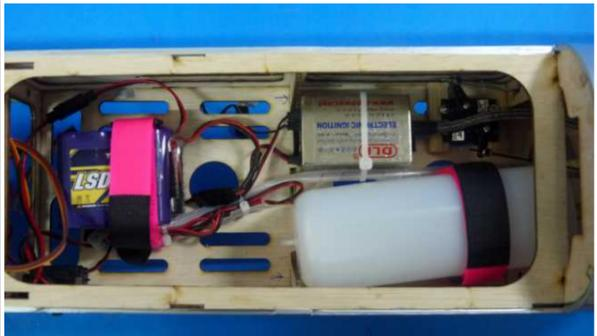
Use Velcro tape to secure the tank and receiver inside in fuselage.
