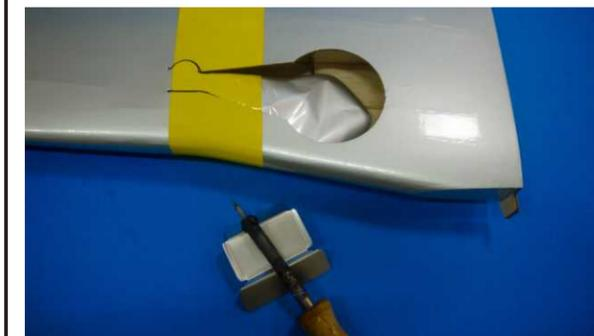
Remove the covering out of the main gear mount.
