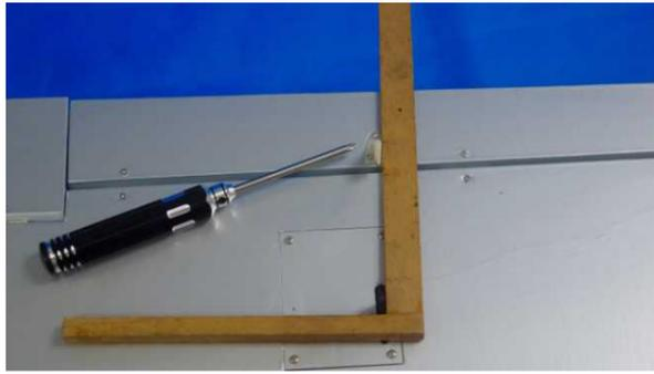
Place the triangle rule along the servo arm to the trailing edge for setting the location for installing the control horn on the aileron. Use 1.5mm hand drill to drill holes for the control horn. Place the control horn in position and the strap on its back and secure with M2x25mm screws.
