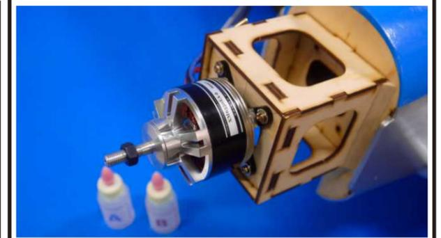
Use Epoxy to secure the motor mount on the fuselage and reinforcing blocks on two sides of motor mount.
