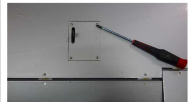
Secure the servo cover in place with M2.6x8 tapping screws.
