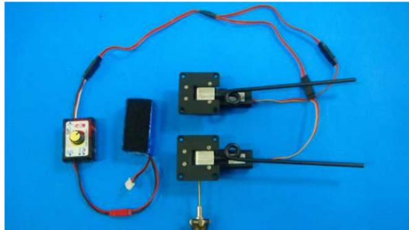
Caution: left main gear is different from right main gear. For identification, please set the gear up, secure the gear to retracts with M3x8 hex screws (the flat side of the gear must face the side screw holes of retract).
