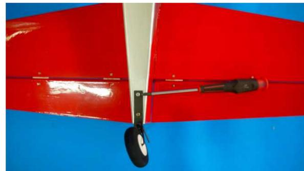
Secure the tail wheel to the tail gear. Use M3x10 tapping screws to secure the tail gear mount to the tail.
