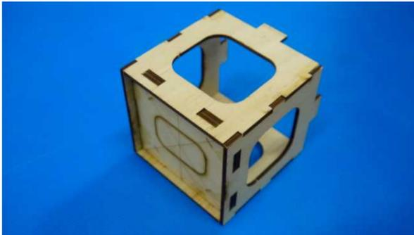
Remove every part out of planking and assemble the parts into motor mount. Use instant glue to secure the parts.
