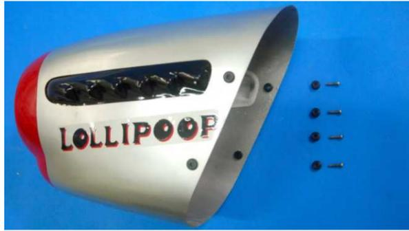
Installing the anti-vibration rubber inside the cowl. Try to fit the cowl to the motor or engine. When satisfy the location, use M2.6x12 tapping screws to secure the cowl in position.
