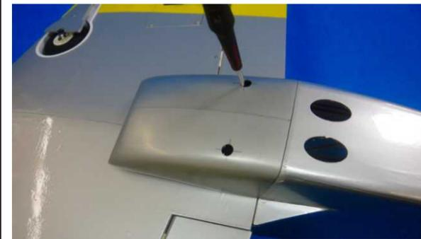
Secure the wing bolts for temporary until the epoxy is dried enough.
