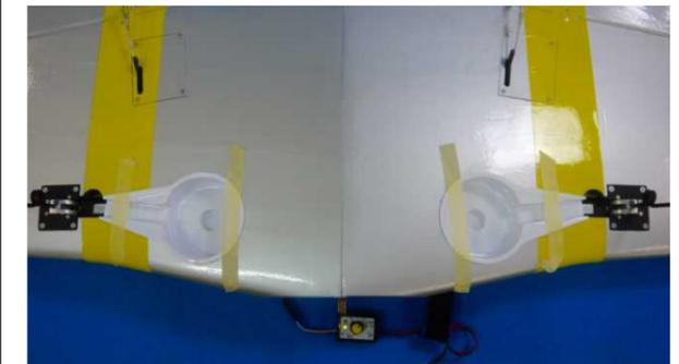
Turn on the power and set the gear down. Install the vacuum-formed mounts for wheels on the main wing and secure them in place with instant glue.
