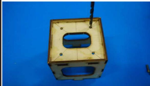
Try to fit the motor onto the motor mount. When satisfy the location, use marker to mark the position for the screws. Remove the motor and use hand drill to open holes on the marked positions.
