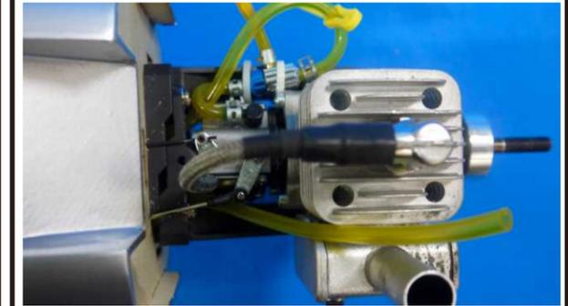
Diagram for assembling the tubing and linkage of the engine.
