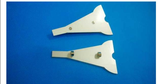
Use M3x6 flat-head screws to secure the collars on the wheel covers for temporary. Don't screw too tight.
