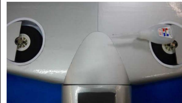
Try to place the aerodynamics on the leading edge of the center main wing. Use instant glue to secure it in place.
