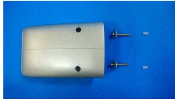
Place the venting M4x35 wing bolts (hex), washers and silicone tubes on the working table.
