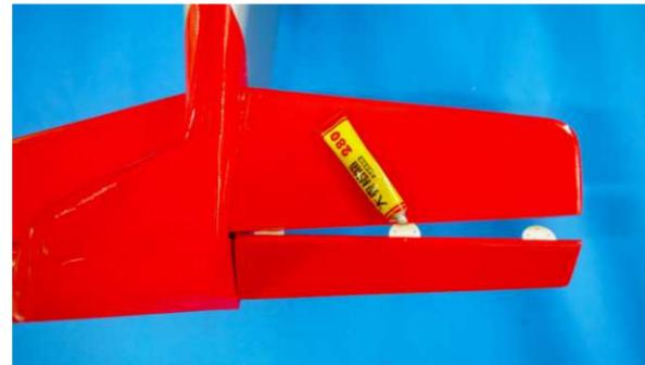
Use Super glue to secure the hinges inside the hinges slot of elevator. Also use Super glue to secure the half of hinges to the horizontal.
