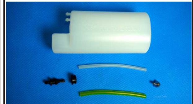
Please take the picture as a reference and assemble the fuel tank combination. If equip with **gas** engine, please select the **yellow** fueling tube.
