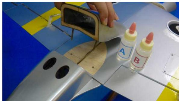
Insert the wing bolts and washers through the venting. Try to fit the vent onto the main wing with the wing bolts into the bolt holes.
