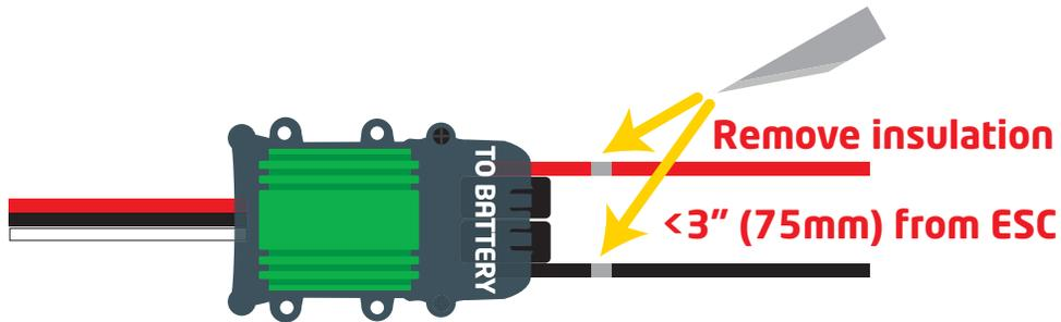
Remove 0.25 inches of insulation from the ESC's power wires within 3 inches of the ESC.
