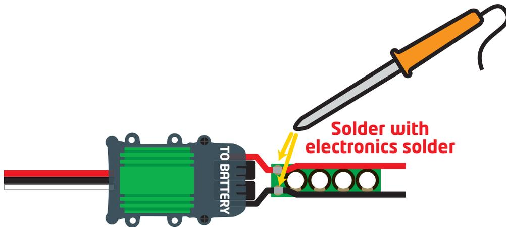
Solder the exposed power wires to the CC CapPack's posts using a high-power iron and electronics solder. Ensure that the RED wire is soldered to the (+) side and the BLACK wire is soldered to the (-) side.
