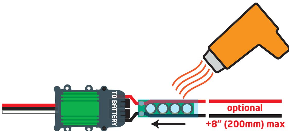
Slide the heat shrink over the CC CapPack and use a heat gun to shrink it. Up to 8 inches of additional wire may be added to the ESC wires.
